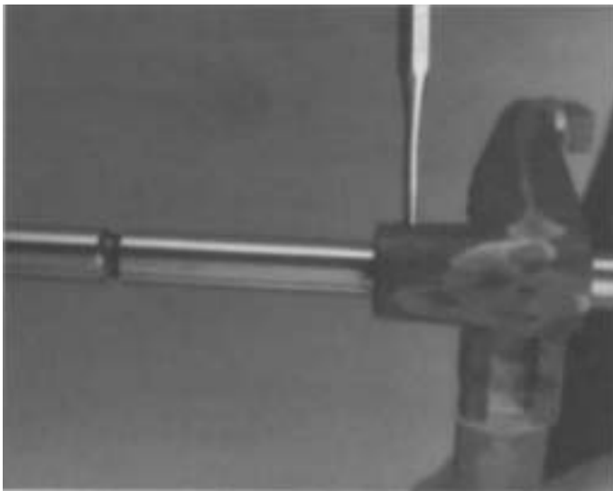
11. If it is necessary to replace yoke or shift blocks, secure shift rail in a vice equipped with brass jaws or wood blocks. Drive the roll pin from yoke and yoke bar as shown.
