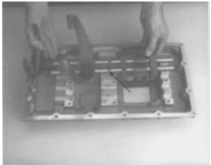
9. Place the reverse, first-second shift bar assembly into the shift bar housing. Check the first-second shift bar to make sure interlock pin is in its proper location (arrow).
