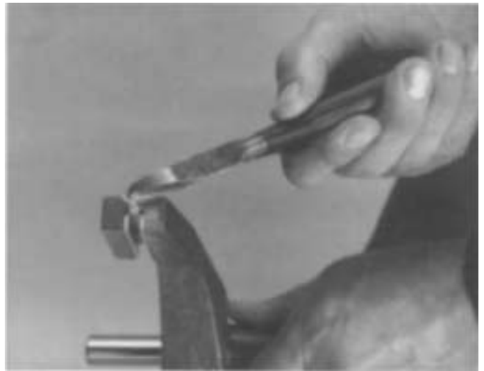
12. If necessary the shift yoke bushings can be replaced. Use pliers to bend the bushing tabs straight then pull the bushings from the yoke slot.
